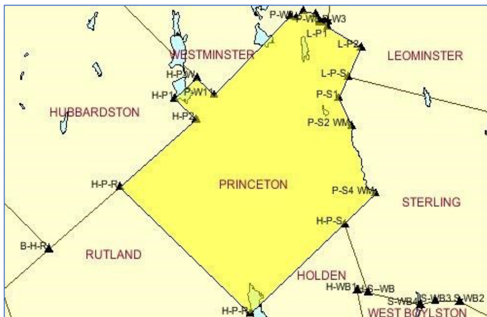
Shows Brian's stone designations at each of the bearing changes of Princeton's boundaries. At each of these points that is a monument.
